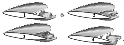
Fig. 16 Fluctuations of the cavity shape ( V_{ref}=6 m/s, \alpha=7 deg, \sigma=0.55 ). ( 30 < T/T_{ref} < 32 , 0.5T_{ref} between two pictures.)
